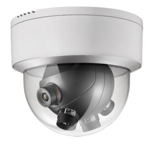
The DarkFighter Series ultra-low light Smart cameras are able to capture high quality color images in dim light environments. DS-2CD9686F-H offers full HD resolution with PoE, defog, and 3D DNR to meet a wide variety of applications.
